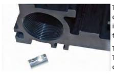
The custom aluminum extrusion is black anodized to resist corrosion. The extrusion is designed to specifically accommodate a linear flow path for each sensor, which is very important for accurate measurement. There are Integrated extruded slots on two faces to allow for "roll-in" t-nuts enabling simple and flexible mounting.
