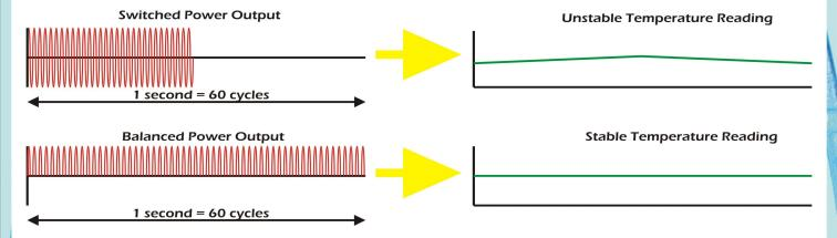
For exceptional mold heater requirements, individual settings of the tuning parameters are available using a combinations of fast, efficient tuning algorithm and balanced power output to the heater, almost any heater is capable of being controlled within 1 degree.
