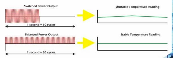
To reduce electrically generated noise, the VISIONS 3000 switches the power to the load as the voltage crosses zero. In addition, the VISIONS 3000 also balances the power output by spreading the ON cycles over a 1 second time period. For example, a 50% output power on other systems consists of half a second with power ON, and half a second with power OFF. With the VISIONS 3000, the power is ON for half a cycle and OFF for half a cycle. As can be seen from the graph above, this produces a
