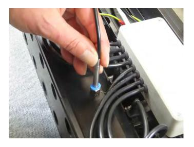
Re-Install the cover back on the manifold
