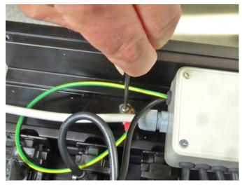
Second - Remove the (2) hex countersunk (M3 x 45) screws from the sensor box
