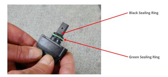
Gently reinstall the sensor in the manifold sensor hole, making sure sealing rings are not pinched. Push down on the sensor, so the sealing rings are tightly seated.
