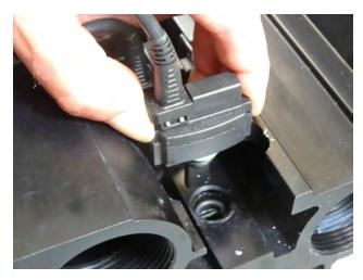
Gently un-snap the wire plug with a small straight screwdriver on each side and gently remove the plug from the sensor.
