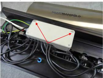
Third - Carefully lift the Sensor Box from the manifold, being careful not to damage or put a strain on wires or apparatus.
