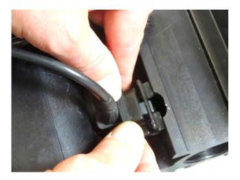
Gently connect the plug, being careful not to bend any of the sensor pins on the socket.
