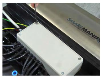
Re-connect the ground wire to the manifold and tighten screw to secure a good ground connection.
