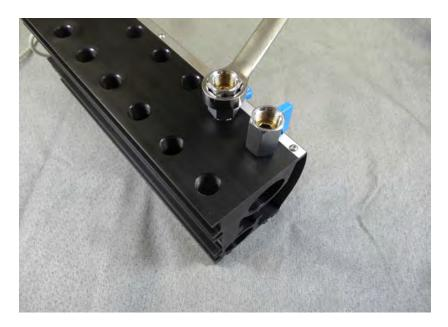
Once all the valves have been installed on the top row, proceed to install the valves on the bottom row.
